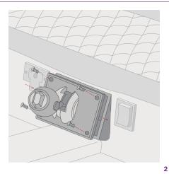
Unscrew the four screws on the shift lever bracket with a screwdriver and remove the Forward-Reverse Shift Lever Assembly (Diagram 1).
