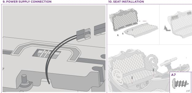
• Securely plug the battery connector into the wire connector.
