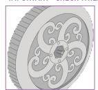
NOTE: If the wheel nuts are loose, the wheels will not engage the forward gear. Tighten the nut with the socket wrench.
